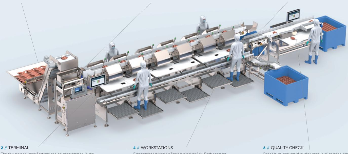
The raw material specifications can be programmed in the system's HMI on the production floor or through the MATRIX PRO software. Operator workstations can be enabled, as well
